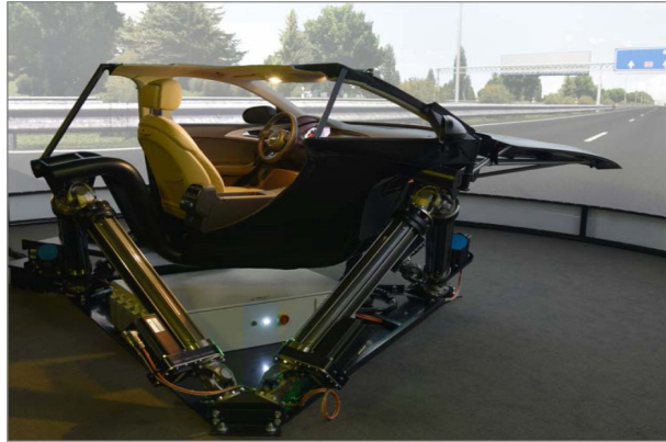
[11] Figure-7: Cruden simulator equipped with a Matlab / Simulink UDP block interface that allows to integrate different vehicle models and other models, such as motion cueing
