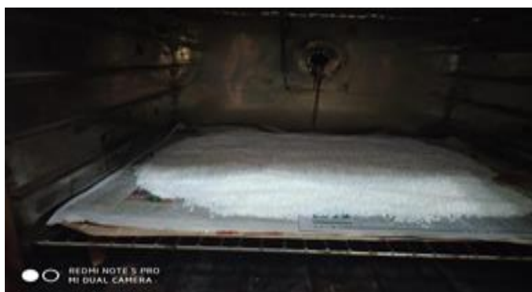
Fig.1 ABS material in hot oven after drying
