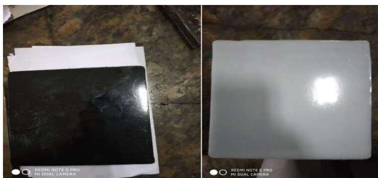
Fig. 2 Preparation of sheets using the compression molding technique
